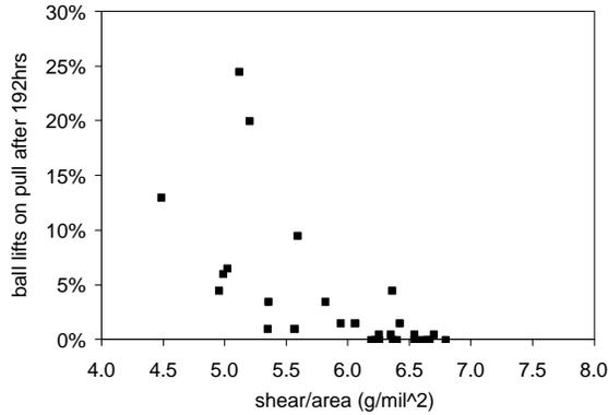
**Figure 14. Pull strength after 192 hrs, 175°C HTS vs. normalized shear strength.**
