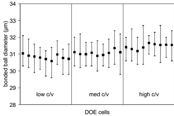
**Figure 1. Bonded ball diameters for the 27 DOE cells.**
