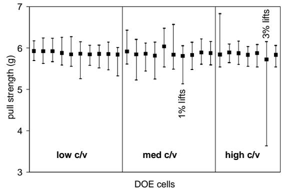
**Figure 4. As-bonded pull strength (above the first bond) for the 27 DOE cells.**
