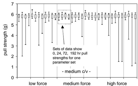
**Figure 8. Pull strength for MEDIUM C/V cells after 175°C HTS.**
