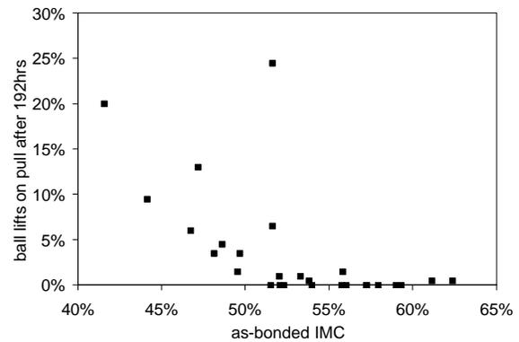
**Figure 17. Ball lift during pull test after 192 hrs, 175°C HTS vs. as-bonded IMC.**
