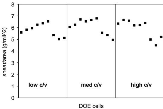
**Figure 3. As-bonded shear strength for the 27 DOE cells.**
