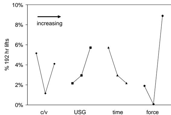
**Figure 13. Ball lifts during pull test after 192 hrs, 175°C HTS vs. bond parameters.**
