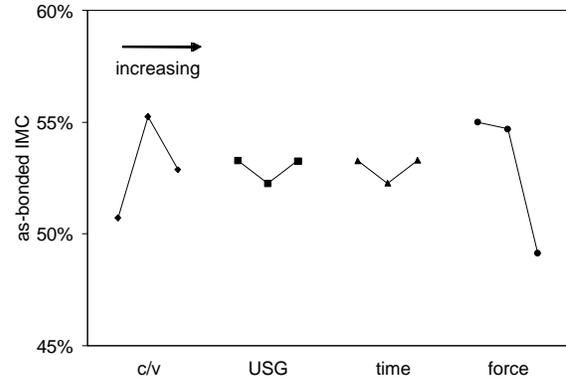
**Figure 11. As-bonded intermetallic coverage vs. bond parameters.**
