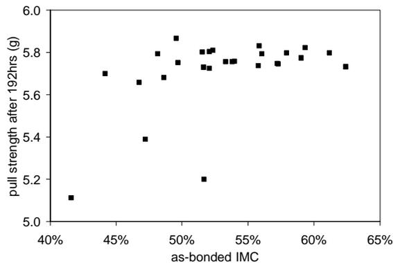
**Figure 15. Pull strength after 192 hrs, 175°C HTS vs. as-bonded IMC.**
