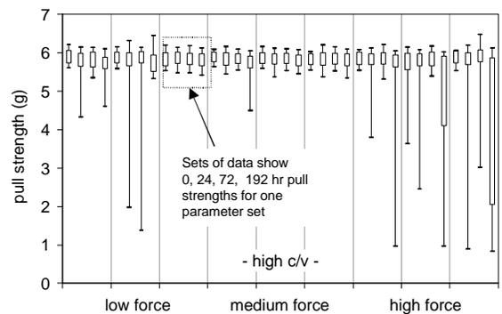
**Figure 9. Pull strength for HIGH C/V cells after 175°C HTS.**
