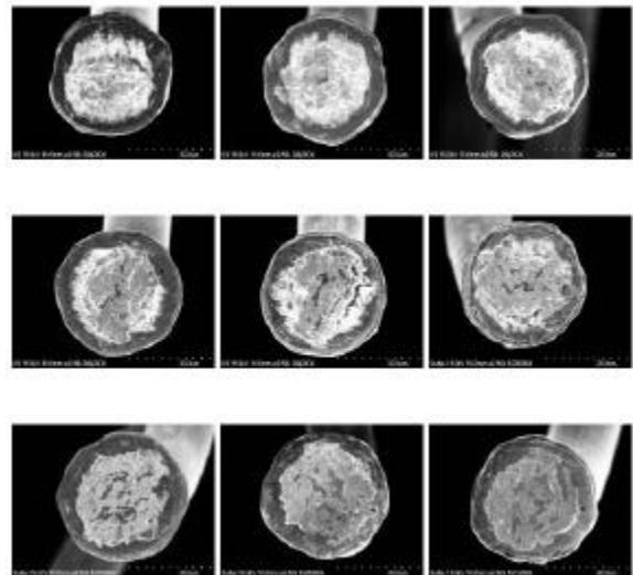
**Figure 5. Example photos of as-bonded intermetallic coverage (IMC) for a sample set using SEM visualization.**
