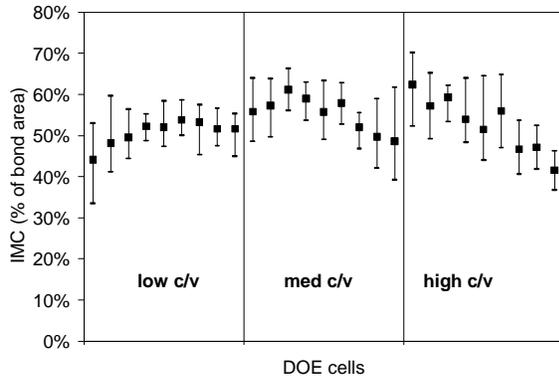
**Figure 6. As-bonded intermetallic coverage (IMC) for the 27 DOE cells (from SEM photographs).**
