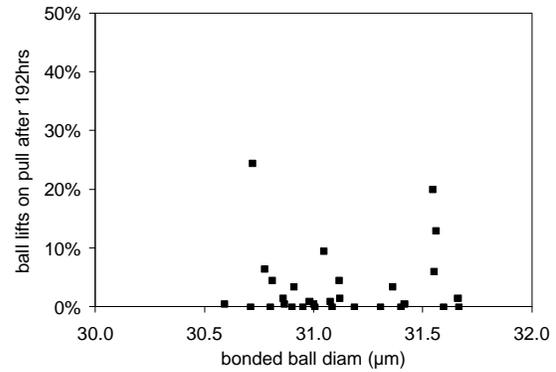
**Figure 16. Ball lifts on pull after 192 hrs, 175°C HTS vs. bonded ball diameter.**
