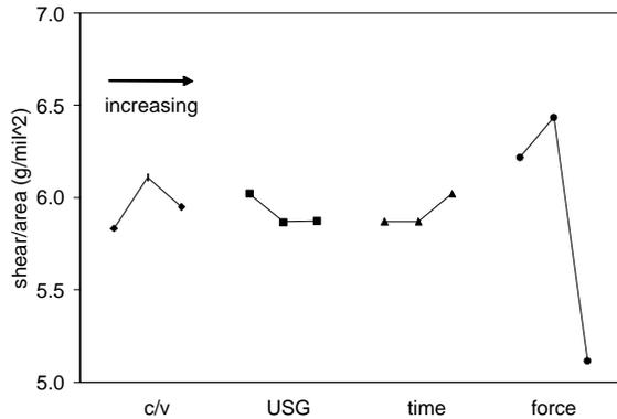
**Figure 10. First bond shear strength vs. bond parameters.**
