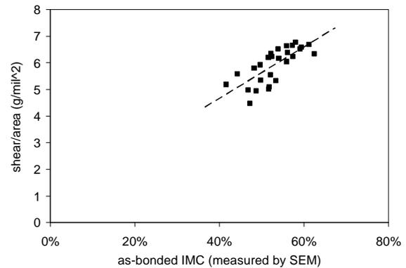
**Figure 12. Normalized shear strength vs. as-bonded IMC.**
