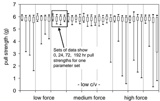
**Figure 7. Pull strength for LOW C/V cells after 175°C HTS.**
