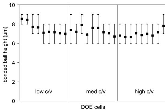
**Figure 2. Bonded ball height for the 27 DOE cells.**
