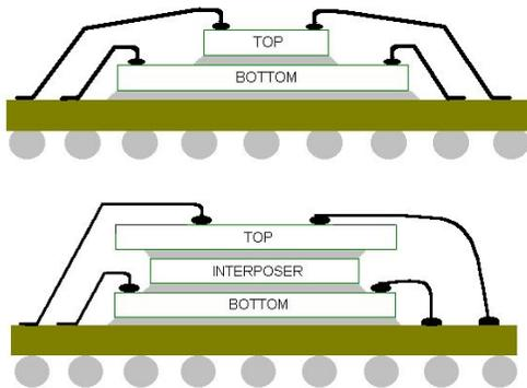
Figure 1 shows examples of the two basic stacked die package configurations: pyramid and cantilevered. Both configurations facilitate die mixing and matching for System-in-Package (SIP) capability. Increasing the cantilever length increases manufacturing flexibility. However, thin, cantilevered die makes manufacturing more difficult. During wire bonding, the cantilever dice deflect and spring back, making bonding difficult to setup and control. Thinned die
