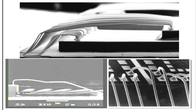
Wire shaping has substantial influence on the productivity of the wire bonding process. In general, each bend adds 10%-20% to the overall wire bond cycle time of the device. Therefore, only the minimum amount of required shaping is recommended for an application. Additionally, excessive shaping can weaken the loop base or neck as well as increase the likelihood of uncontrolled kinking along the wire path.
