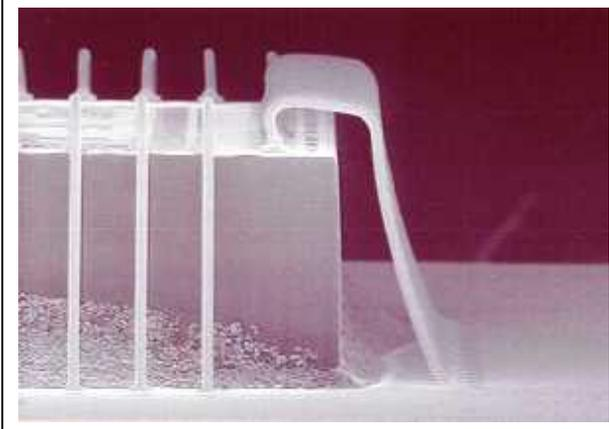
for applications where they must span over lower wire layers in multi-tiered packages. The worked loop has been shown to have superior thermal cycling performance in hermetic applications where the outer kink can absorb the strain of thermal cycling better than the HAZ in a standard loop shape.
