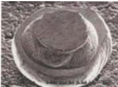
Figure 4: Gold bump after coining
