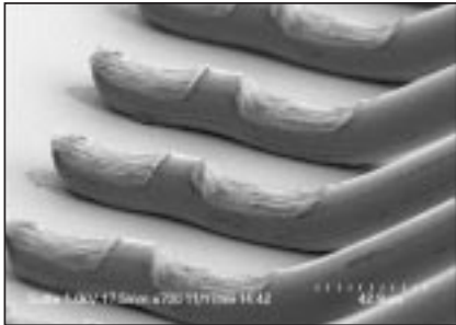
Figure 5. Wedge-bonded copper wires reflect the cross-groove in the tip of the bonding tool that is designed to increase the coupling between the ultrasonic transducer and the wire.
