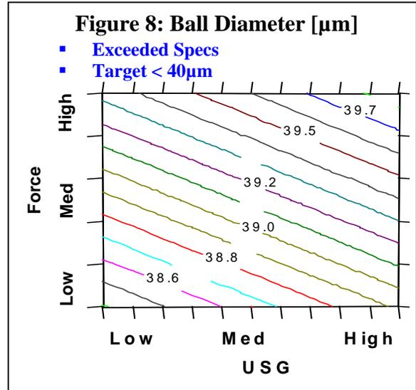
activity that the copper process currently faces. Optimization of these applications, with 20μm wire diameter and 40μm bonded ball diameter, is challenging, even for a gold bonding process. The use of Design of Experiments techniques is necessary to understand the interplay of all of the variables. Figures 7-9 show data from a DOE, optimizing the ball size, shear strength and pull strength.
