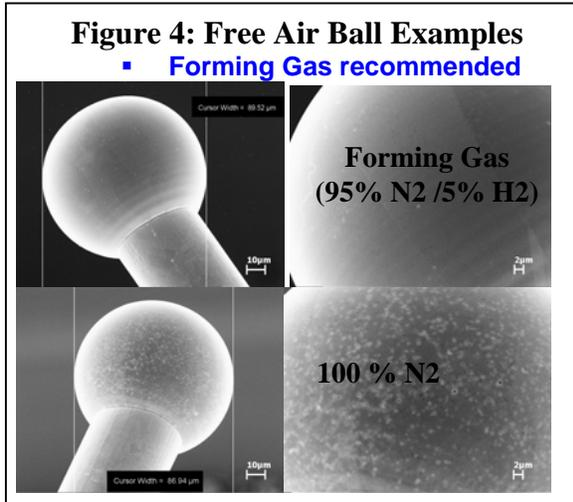
gas provides the best results and is required for devices with advanced, sensitive bond pad metallization, N2 can often provide acceptable results with low I/O, large pitch standard devices. Hydrogen levels greater than 5% are flammable (5% is not a flammable mixture) and are not recommended.
